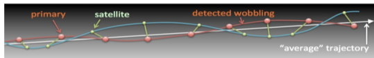
Figure 1 - Schematics of the astrometric method to detect moons around asteroids. The red trajectory is the « signature » of the satellite presence, relative to the unperturbed trajectory (white) that would be followed by the asteroid in the sky.
