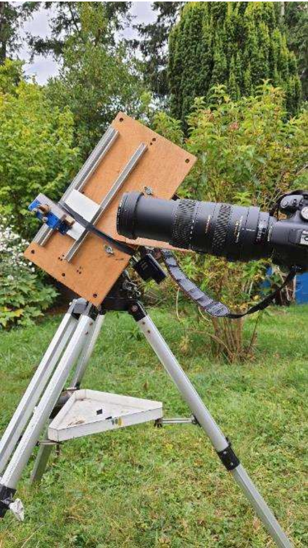
Pupil grating spectrograph demonstrateur using blazed grating 1200 grooves/mm 58mm (Jobin & Yvon Horiba) 400mm zoom lens Pascal Goumard, Thierry Midavaine
