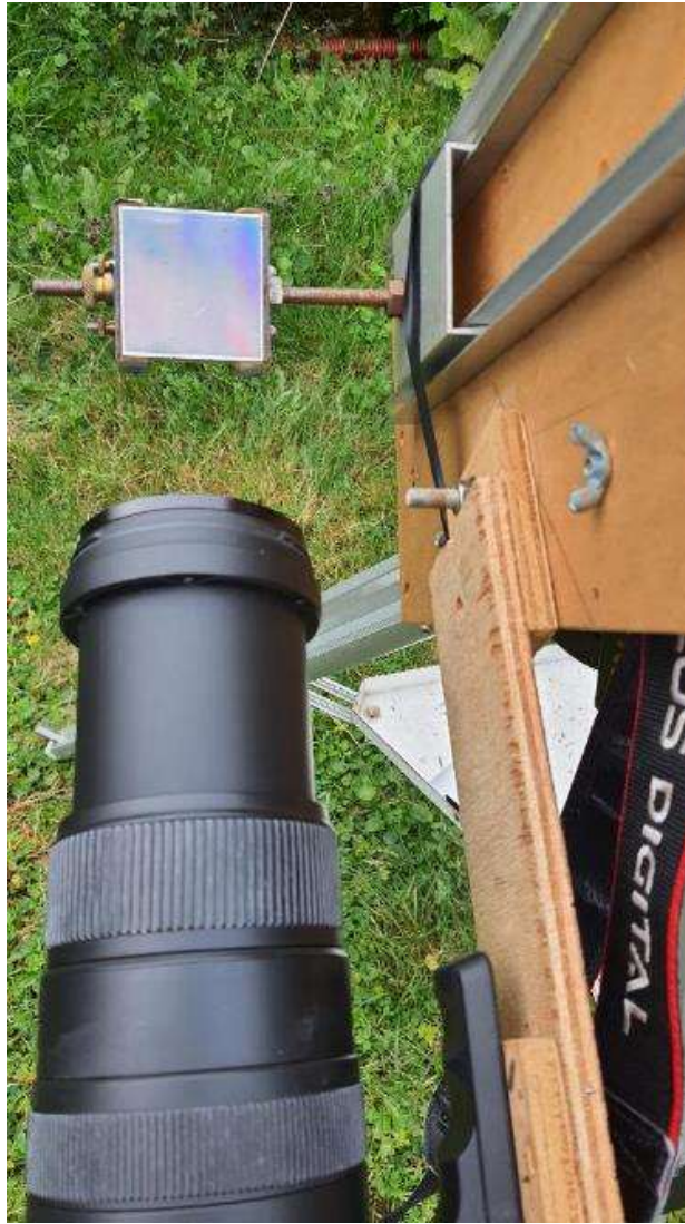
Pupil grating spectrograph demonstrateur using blazed grating 1200 grooves/mm 58mm (Jobin & Yvon Horiba) 400mm zoom lens Pascal Goumard, Thierry Midavaine
