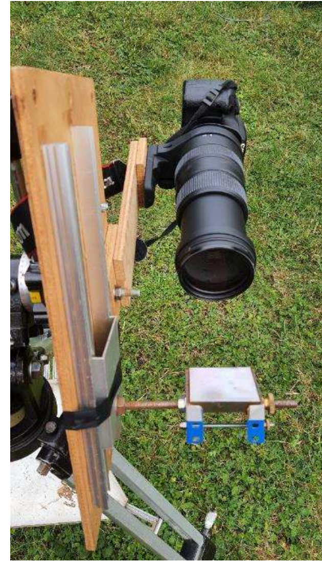
Pupil grating spectrograph demonstrateur using blazed grating 1200 grooves/mm 58mm (Jobin & Yvon Horiba) 400mm zoom lens Pascal Goumard, Thierry Midavaine
